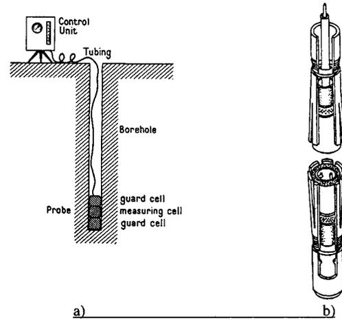
**FIG. 1 a) Basic Principles of the Triple Cell Design Pressuremeter (Baguelin, Jézéquel and Shields, 1978,<sup>3</sup> b) Slotted Tube with Probe**
