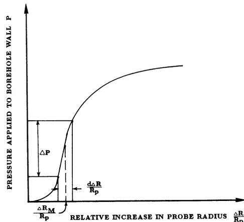
FIG. 9 Pressure Versus Relative Increase in Radius
