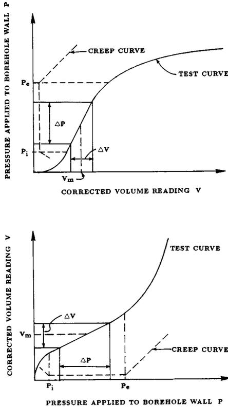
FIG. 8 Pressuremeter Test Curves for Procedure A
