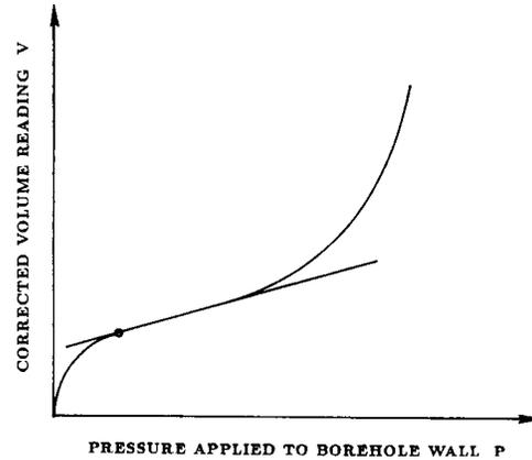
FIG. 4 Ideal Shape of the Pressuremeter Corrected Curve
